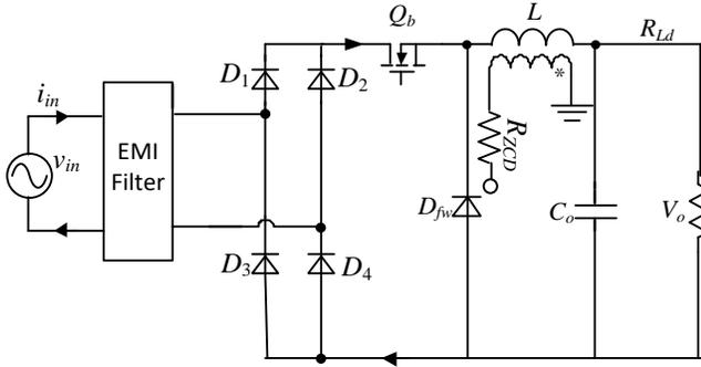
Fig.1 Schematic diagram buck converter
