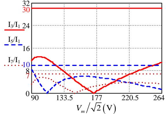
Fig. 7 Contents of input current harmonic along with limits
