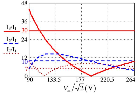
Fig. 3 Contents of input current harmonic along with limits
