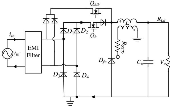
Fig. 5 Schematic diagram of introduced topology
