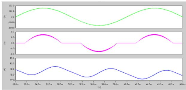
Figure 8  $v_{in}$ ,  $i_{in}$ , and  $v_o$  for buck converter
