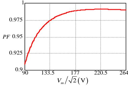
Fig. 4 Input PF for CRM buck converter
