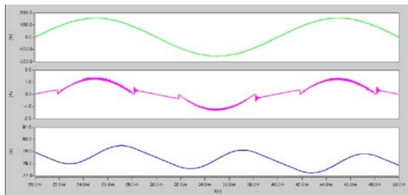
Fig.9  $v_{in}$ ,  $i_{in}$ , and  $v_o$  for buck-buck/boost converter
