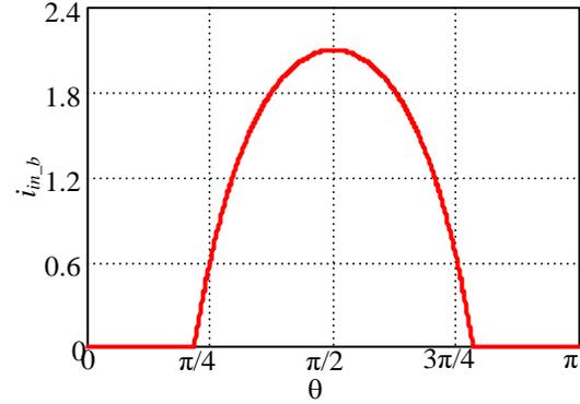
Fig. 2 Input current of CRM buck PFC converter
