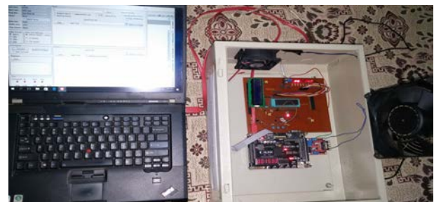
Fig. 4 The System on Chip showing the ADC module PCB
