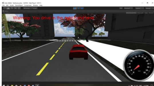
Fig. 13 Simulation System warns “Getting in the right-hand lane”
