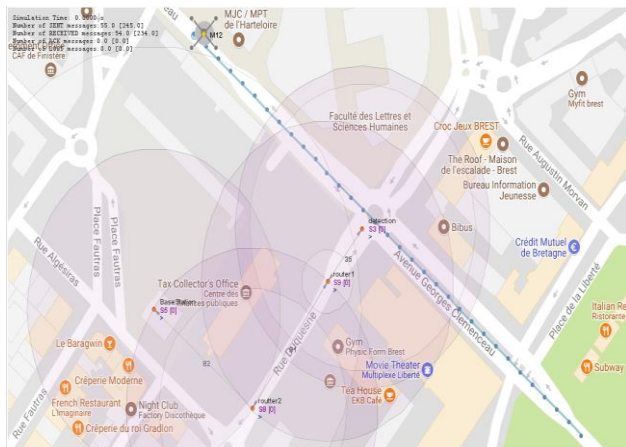
Fig. 8 (a). Sensors are not sensing any vehicle in TMS-SC simulation
