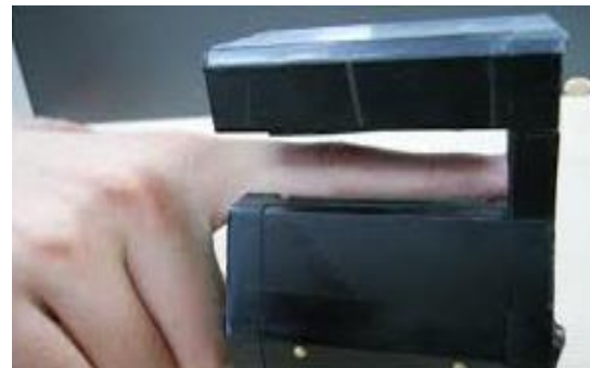
Fig. 2 The Finger-veins capturing device [15].
