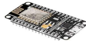
Fig. 7 ESP8266 modules used for the experiment
