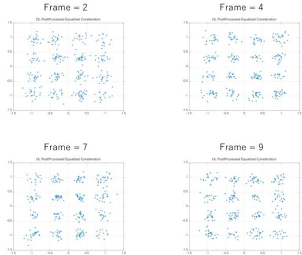
Fig. 10 Simulation results of Resample, De-rotate, Phase compensation are ON.
