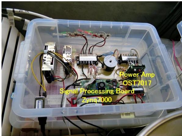
Fig. 17 Zynq7000 ARM-embedded FPGA is used for digital signal processing and OST7010 Power Amplifier drives TX transducer through transformer.
