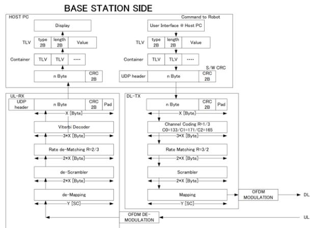
Fig. 15 Block diagram of Base Station side system.
