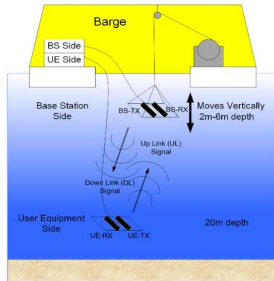
Fig. 11 Ocean Experiment to check Robust TDD synchronization.
