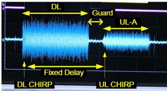
Fig. 13 Measured TDD waveform.
