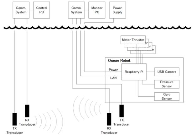
Fig. 18 Block diagram of the prototype ocean robot system.
