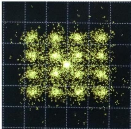
Fig. 14 Demodulated 16QAM constellation at UE-RX side
