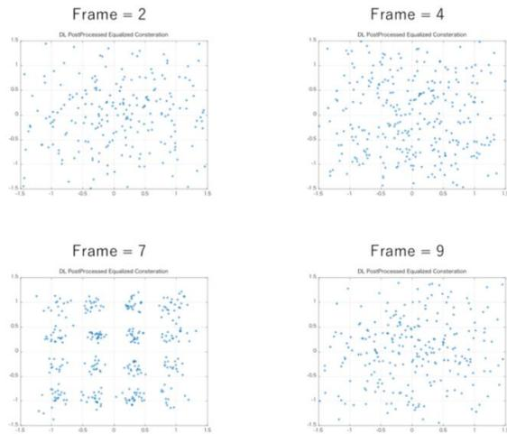
Fig. 9 Simulation results of Resample, De-rotate, Phase compensation are OFF.
