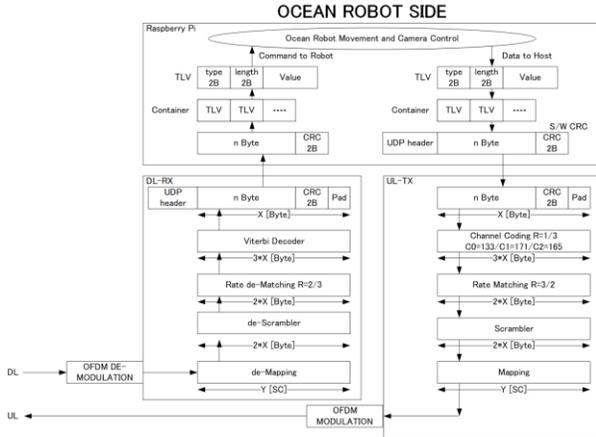
Fig. 16 Block diagram of Robot side system
