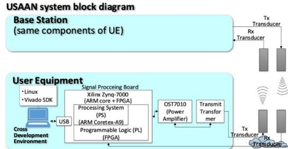
Fig. 6 USAAN implemented target system block diagram.
