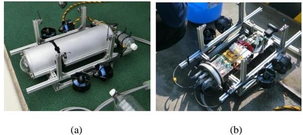
Fig. 19 Underwater Robot with cover (a) and without cover (b).
