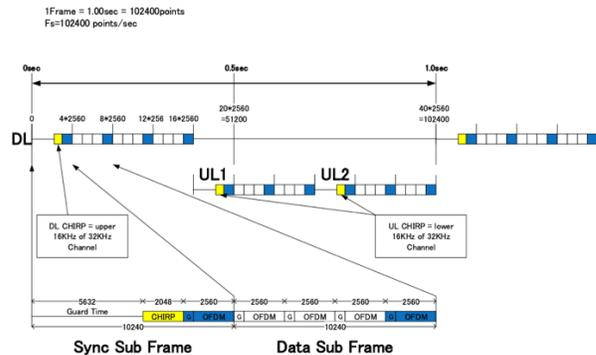
Fig. 4 Frame Design of USAAN system.
