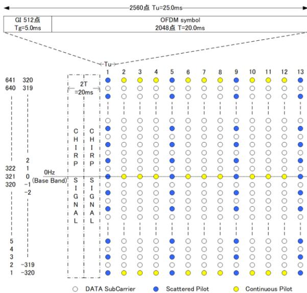
Fig. 5 Time-Frequency Diagram of USAAN system.
