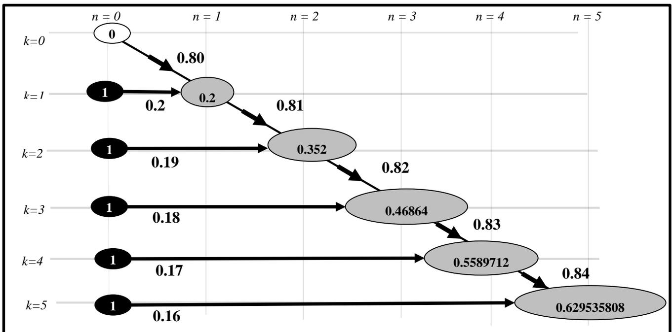
Fig. 13. Actual computations implemented on the SFG of Fig. 7 to obtain the expectation  $E\{s\{< 3\}\}(5, 5, p\{\geq 3\})$  of system failure at level 3. Every node value in the figure is complementary to the corresponding node in Fig. 12. This kind of unreliability computation is not recommended for the present series system (but is preferable for a parallel system).
