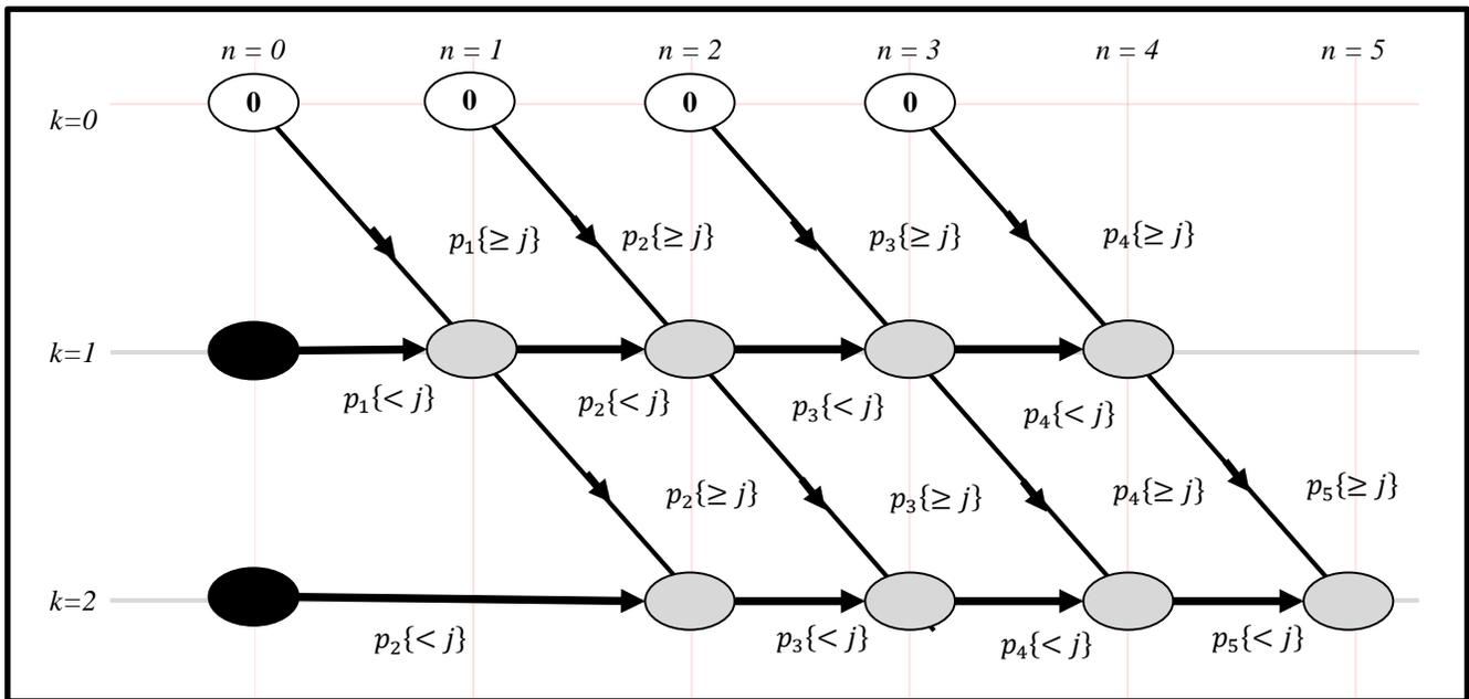
FIG. 5. A SIGNAL FLOW GRAPH IMPLEMENTING THE UNRELIABILITY VERSION OF THE AR ALGORITHM FOR COMPUTING THE EXPECTATION  $E\{s\{< j\}\}(2, 5, \mathbf{p}\{\geq j\})$  OF SYSTEM FAILURE AT LEVEL  $j$  WHEN  $k_j = 2$  AND  $n = 5$ . EVERY NODE VALUE IN THE FIGURE IS COMPLEMENTARY TO THE CORRESPONDING NODE VALUE IN FIG. 2.
