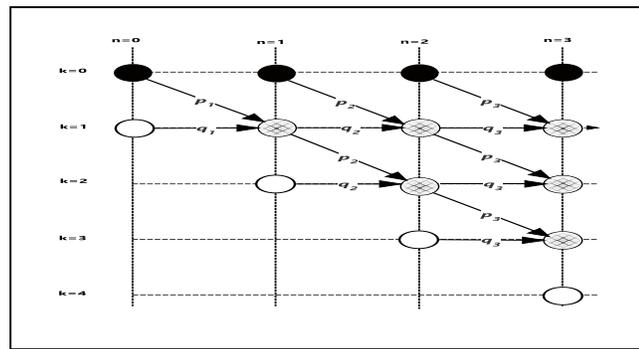
Fig. 1. A Mason signal flow graph that illustrates the computation of the reliability  $R(k, n, \mathbf{p})$  of a binary k-out-of-n system.
