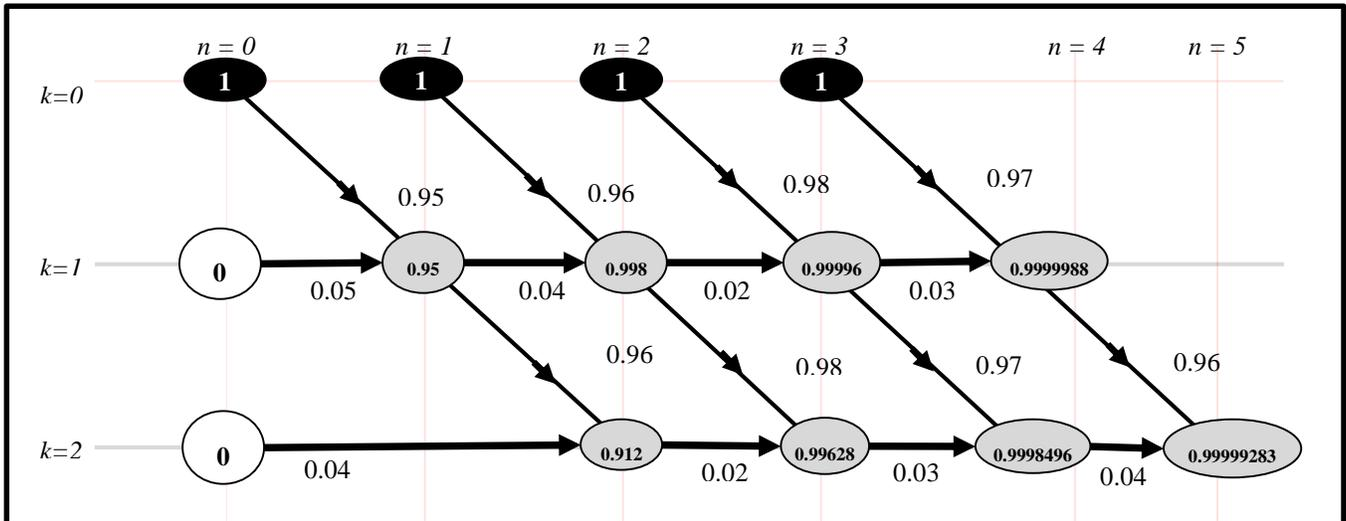
Fig. 8. Actual computations implemented on the SFG of Fig. 2 to obtain  $E\{s\{\geq 1\}\}(2, 5, p\{\geq 1\})$  of system success at level 1. The figure manifests the inconvenience of representing ultra-reliabilities in fixed-point format.
