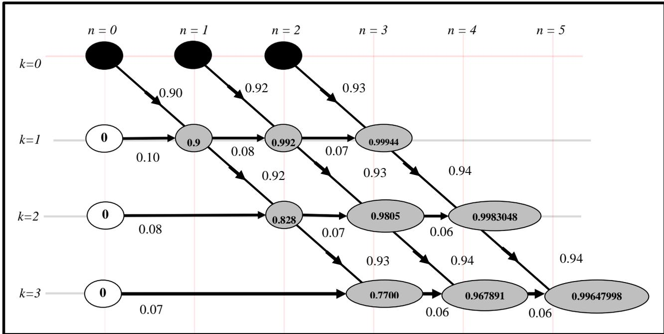
Fig. 10. Actual computations implemented on the SFG of Fig. 3 to obtain  $E\{s\{\geq 2\}\}(3, 5, p\{\geq 2\})$ . Again, the figure manifests the inconvenience of representing ultra-reliabilities in fixed-point format.
