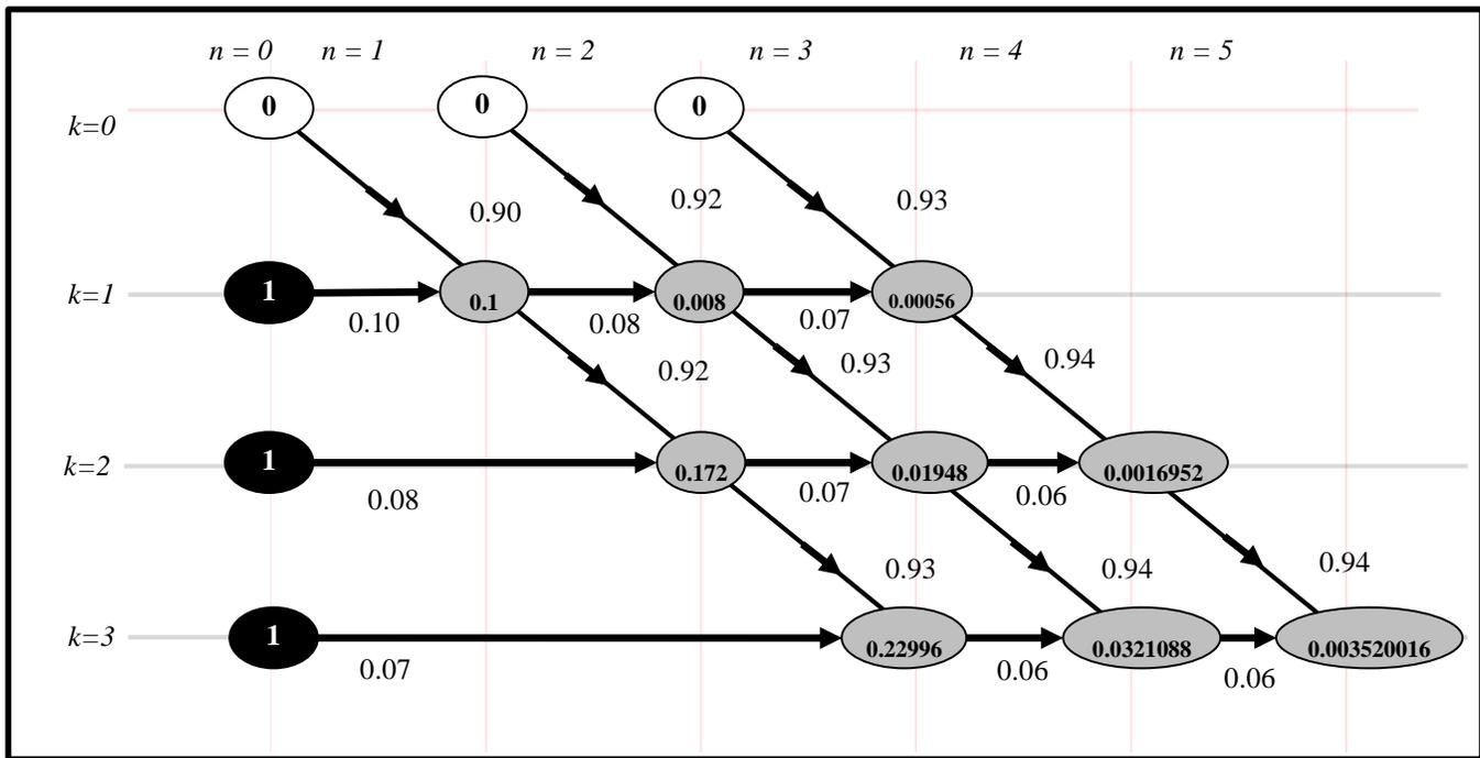
Fig. 11. Actual computations implemented on the SFG of Fig. 6 to obtain the expectation  $E\{s\{< 2\}\}(2, 5, p\{\geq 2\})$  of system failure at level 2. Again, the figure demonstrates the numerical convenience of dealing with probability of failure rather than that of success when dealing with ultra-reliable systems. Every node value in the figure is complementary to the corresponding node value in Fig. 10.
