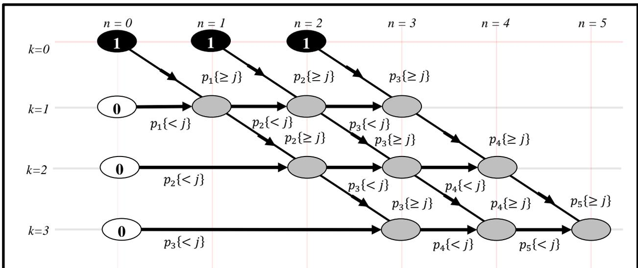
Fig. 3. A signal flow graph implementing the reliability version of the AR algorithm for computing the expectation  $E\{s\{\geq j\}\}(3, 5, \mathbf{p}\{\geq j\})$  of system success at level  $j$  when  $k_j = 3$  and  $n = 5$ .
