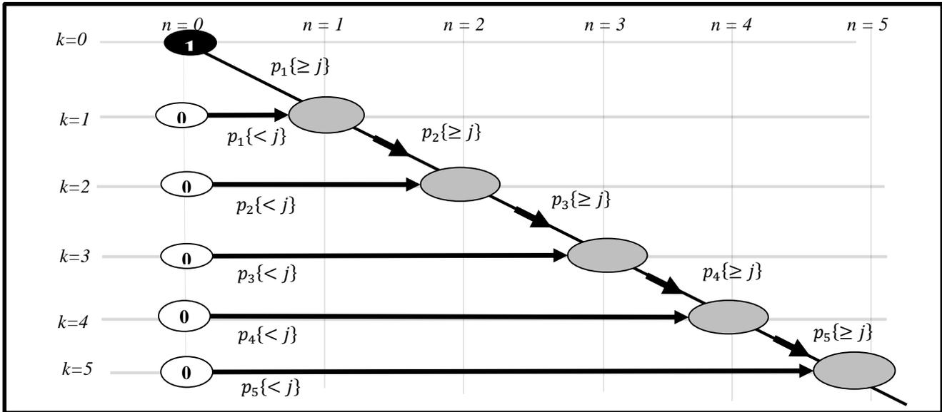
Fig. 4. A signal flow graph implementing the reliability version of the AR algorithm for computing the expectation  $E\{s\{\geq j\}\}(5, 5, \mathbf{p}\{\geq j\})$  of system success at level  $j$  when  $k_j = 5$  and  $n = 5$ .
