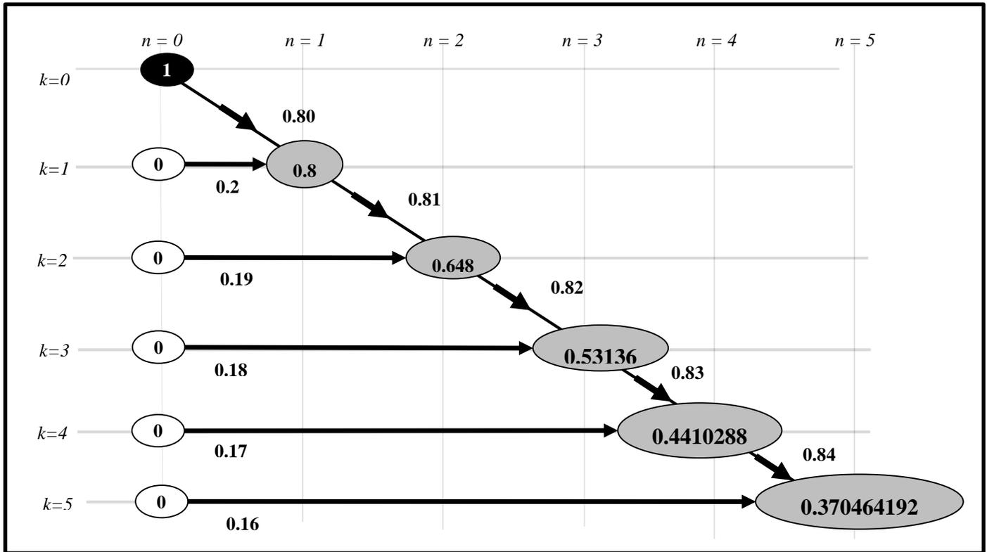
Fig. 12. Actual computations implemented on the SFG of Fig. 4 to obtain  $E\{s\{\geq 3\}\}(5, 5, p\{\geq 3\})$ . This reliability figure neatly recovers the celebrated reliability-product formula of a series system. Dually, the unreliability version of the AR algorithm is equally efficient in obtaining the dual (albeit much less known) unreliability-product formula of a parallel system.
