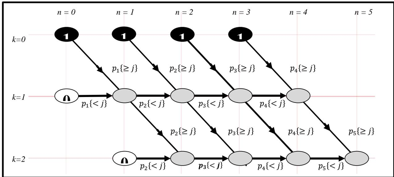
Fig. 2. A signal flow graph implementing the reliability version of the AR algorithm for computing the expectation  $E\{s\{\geq j\}\}(2, 5, \mathbf{p}\{\geq j\})$  of system success at level  $j$  when  $k_j = 2$  and  $n = 5$ .
