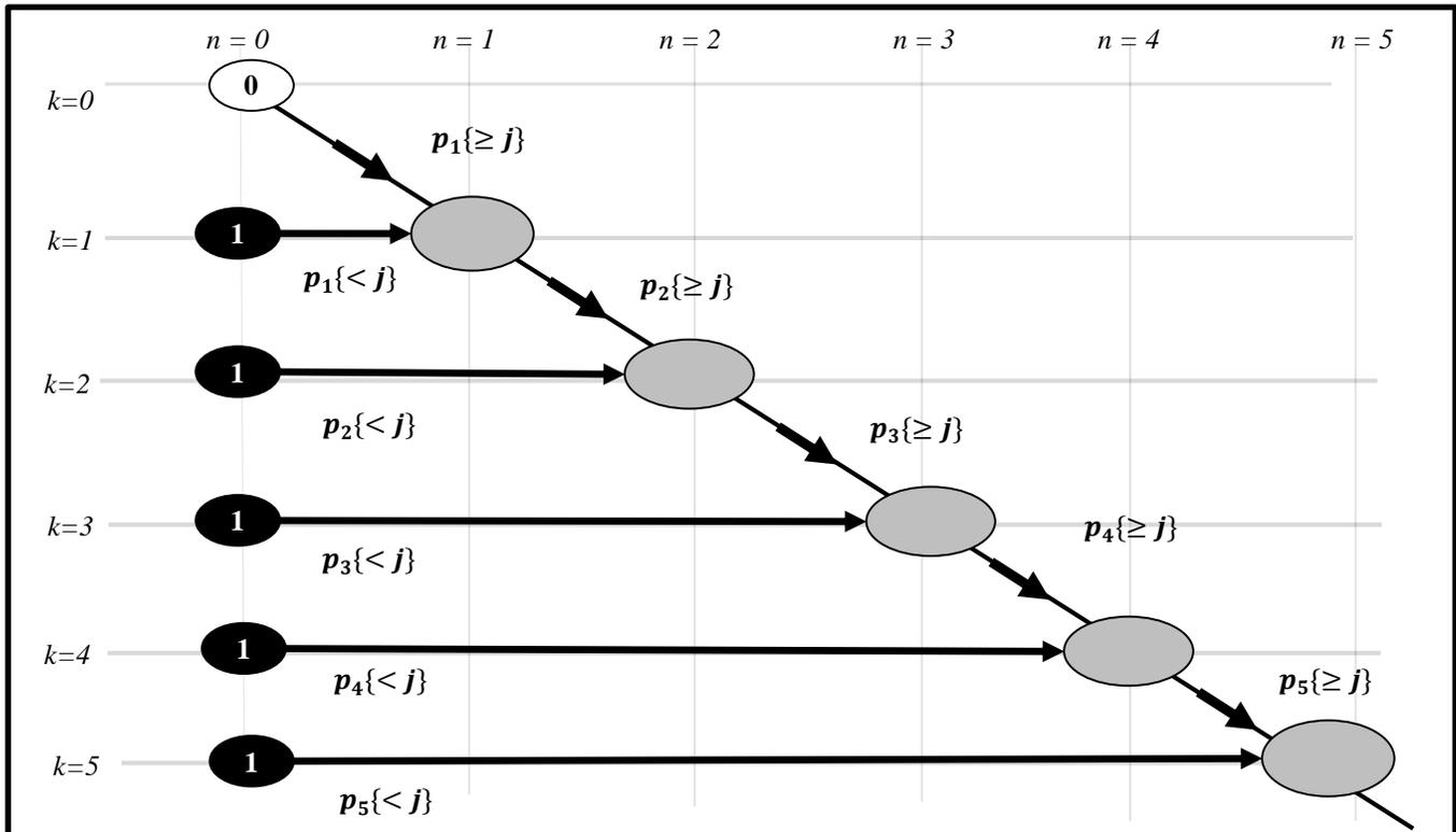
Fig. 7. A signal flow graph implementing the unreliability version of the AR algorithm for computing the expectation  $E\{S\{< j\}\}(5, 5, p\{\geq j\})$  of system failure at level  $j$  when  $k_j = 5$  and  $n = 5$ . Every node value in the figure is complementary to the corresponding node value in Fig. 4.
