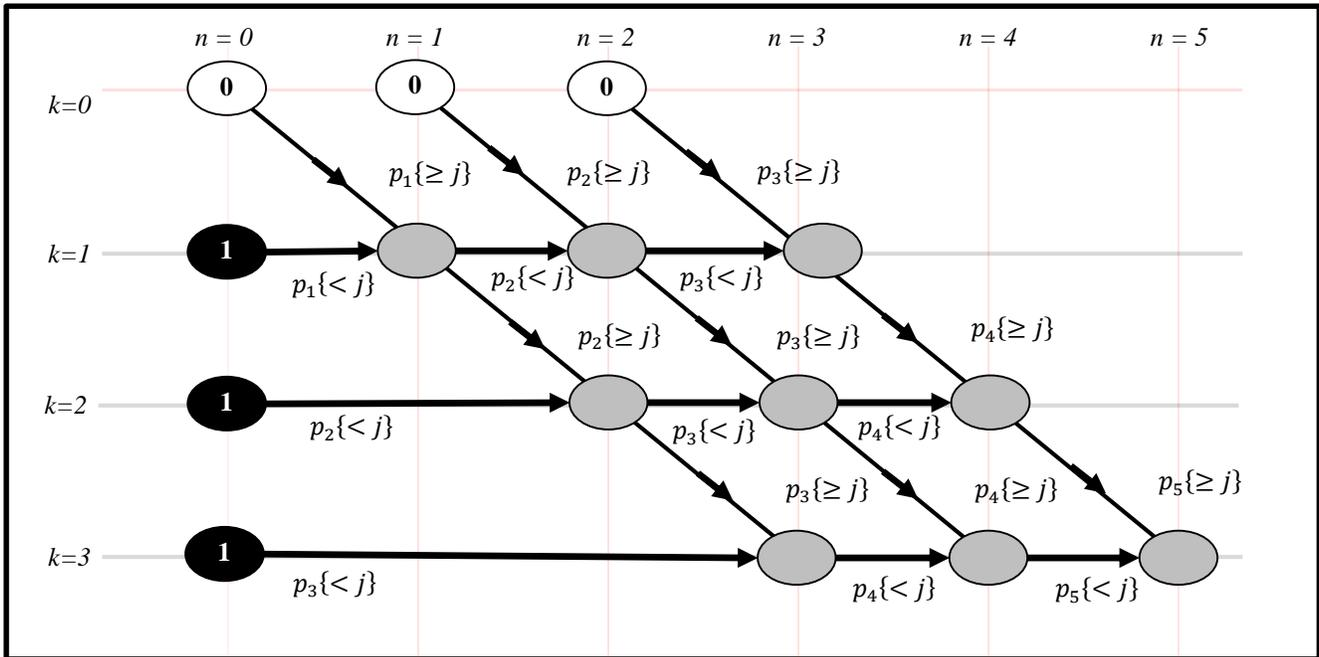
Fig. 6. A signal flow graph implementing the unreliability version of the AR algorithm for computing the expectation  $E\{s\{< j\}\}(3, 5, p\{\geq j\})$  of system failure at level  $j$  when  $k_j = 3$  and  $n = 5$ . Every node value in the figure is complementary to the corresponding node value in Fig. 3.
