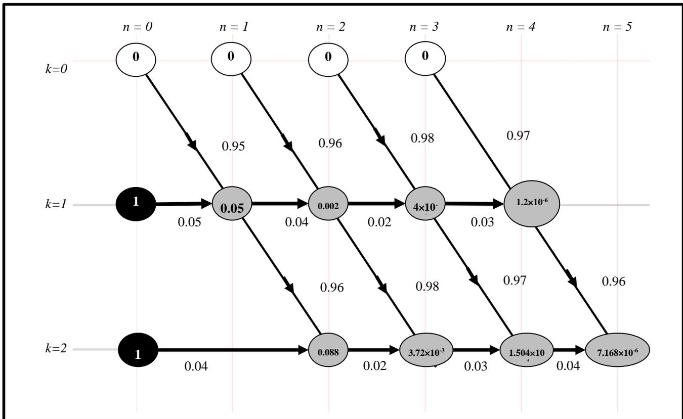
Fig. 9. Actual computations implemented on the SFG of Fig. 5 to obtain the expectation  $E\{s\{< 1\}\}(2, 5, p\{\geq 1\})$  of system failure at level 1. The figure demonstrates the numerical convenience of dealing with probability of failure rather than that of success when dealing with ultra-reliable systems. Every node value in the figure is complementary to the corresponding node value in Fig. 8.
