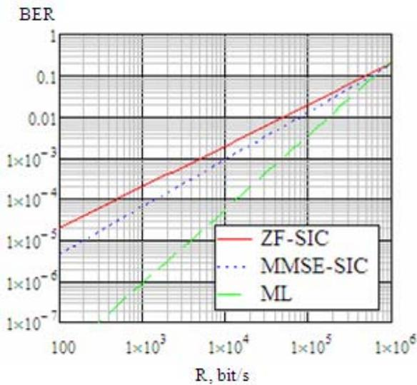
Fig. 4. Dependencies of BER on bit rate for three types of spatial multiplexing
