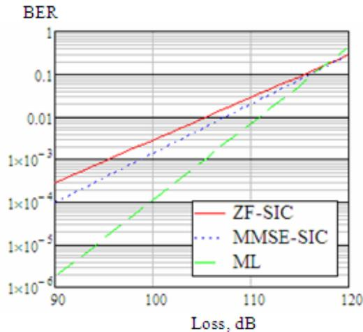
Fig. 3. Dependencies of BER versus losses for different types of spatial multiplexing
