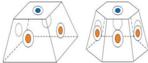
Fig. 1. An example of a configuration for a UV communication module with 4 (left) and 6 (right) narrow directional emitters on the side faces and one wide directional receiver on the top face [20].
