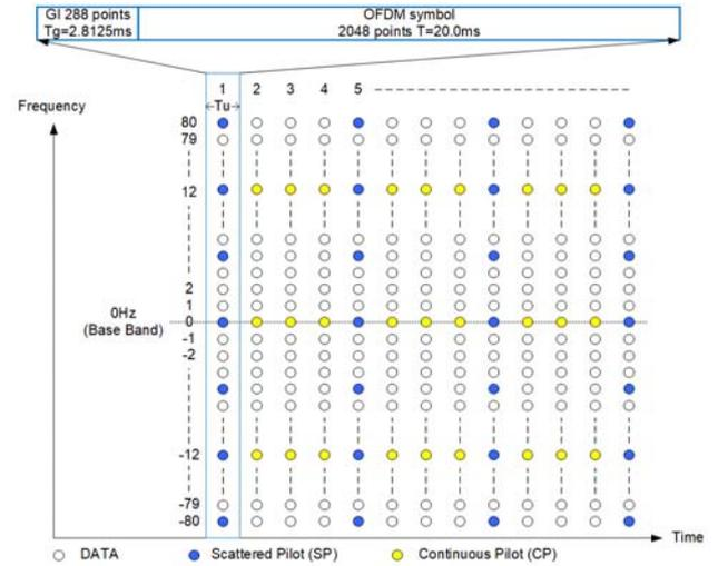
Fig. 4: Time-Frequency structure of OFDM
