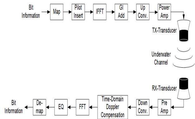
Fig. 2 A Typical UWA OFDM Communication system
