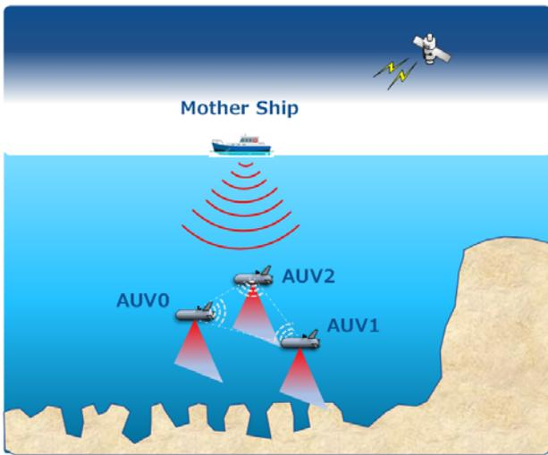
Fig. 1: Swarming AUVs and mother ship for underwater exploration system controlled by UWA communication
