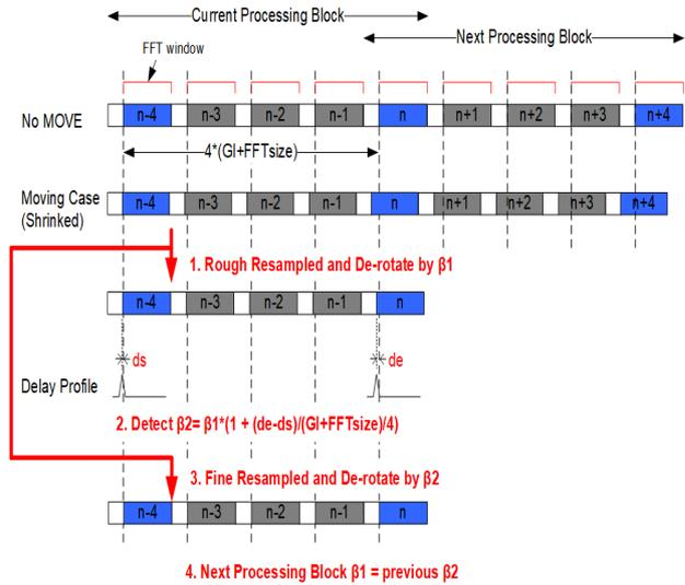
Fig. 8: 2 steps shrink-expansion processing
