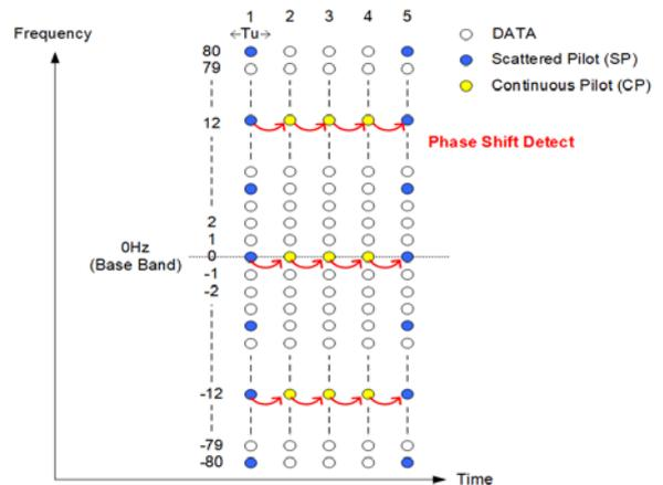
Fig. 10: Frequency-Domain Phase Shift Detection
