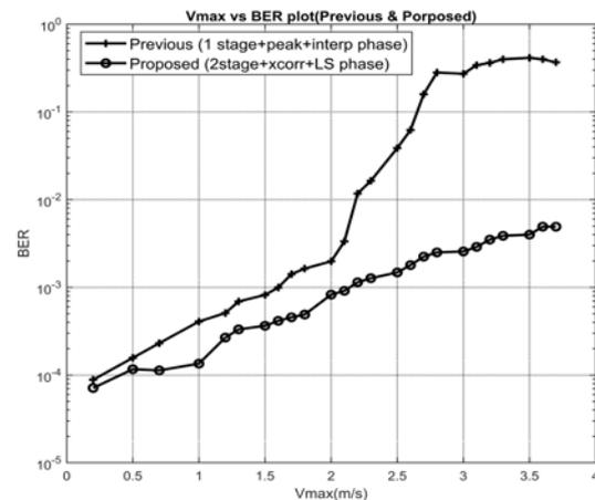
Fig. 14: BER plot of Previous and Proposed algorithm
