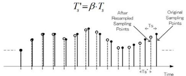
Fig. 7: Resample processing
