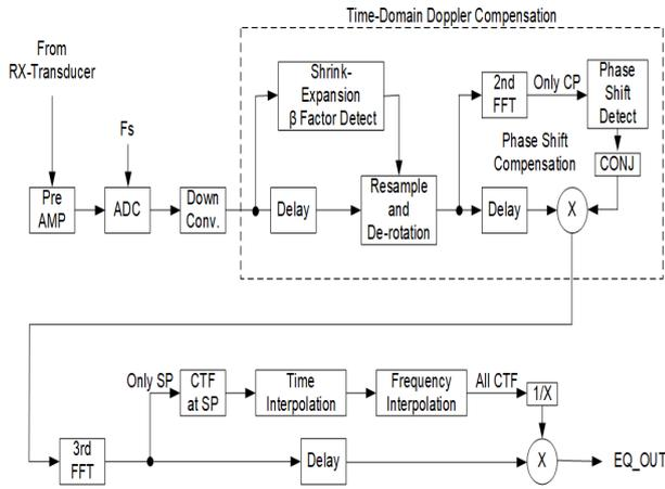
Fig. 3 Receiver Block Diagram
