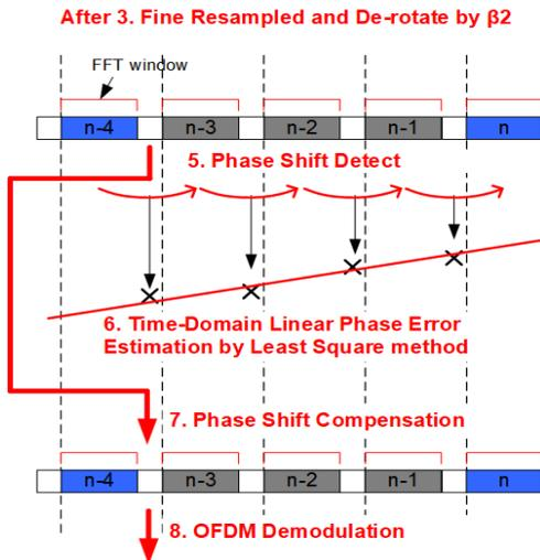
Fig. 11: Phase shift compensation processing
