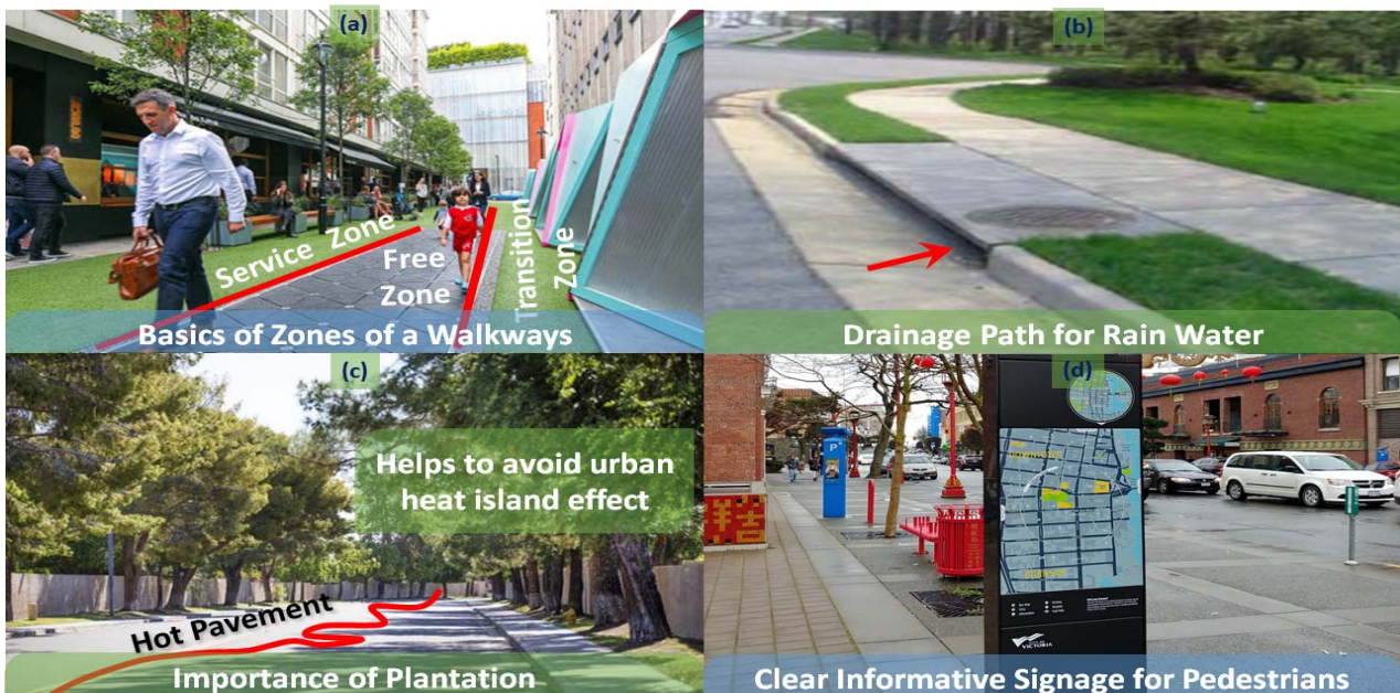
Fig. 1. Some of the key principle parameters of a walkway
