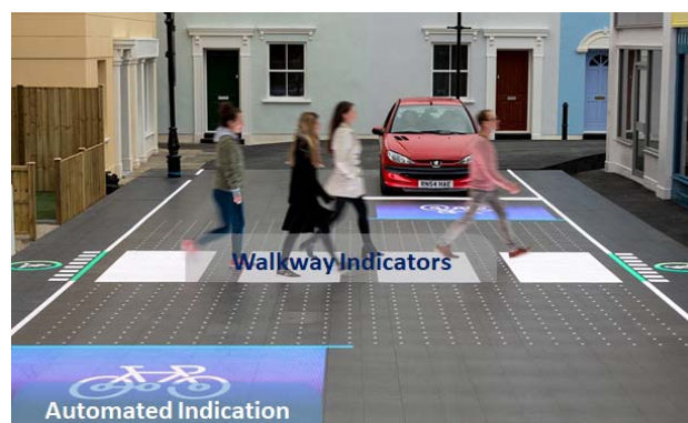
Fig. 4. Interactive floor tile directing the pedestrians over the walkways
