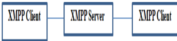
Fig. 6 A simple XMPP architecture with two clients [7]
