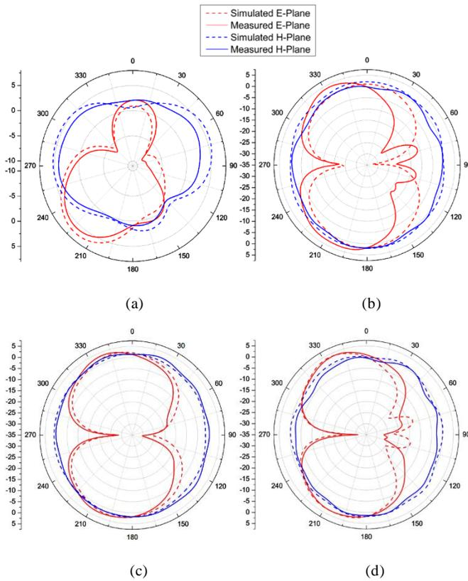
Fig. 10 Measured and simulated radiation patterns at (a) 0.9, (b) 2.1, (c) 2.4 and (d) 2.6 GHz.
