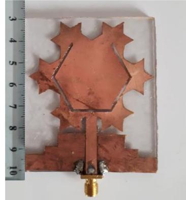
Fig. 8 Fabricated antenna.
