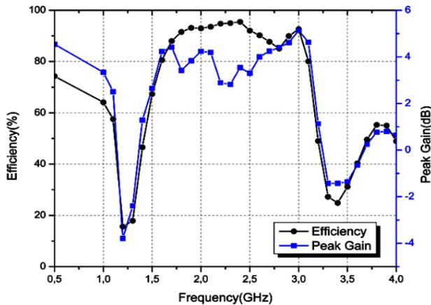
Fig. 11 Measured peak gain and radiation efficiency of the proposed antenna.
