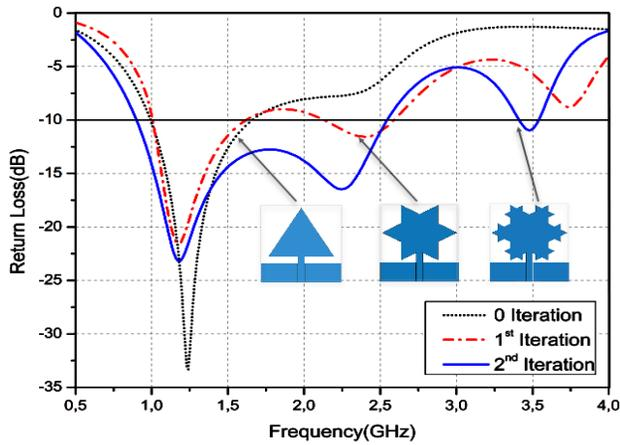
Fig. 3  $S_{11}$  of different iterations of the proposed antenna.
