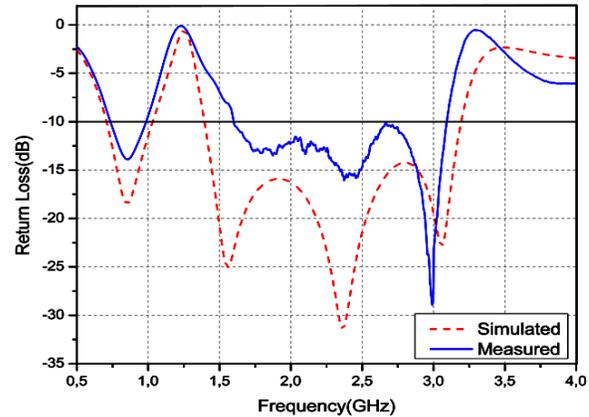
Fig. 9 Measured and simulated reflection coefficient of the proposed antenna.
