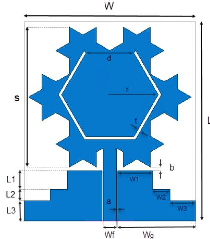
Fig. 2 Fractal antenna geometry.
