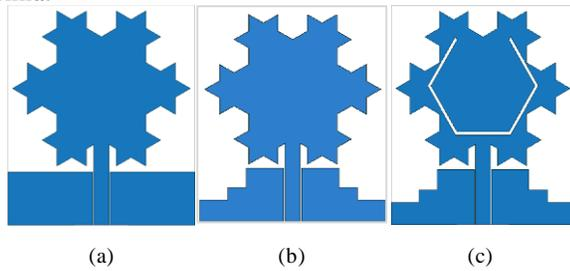
Fig. 4 Evolution steps of the proposed antenna: (a) 2<sup>nd</sup> iteration, (b) 2<sup>nd</sup> iteration + SGP, (c) 2<sup>nd</sup> iteration+SGP+slot.
