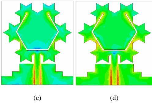
Fig. 6 Current distributions of the proposed fractal antenna at (a) 0.9, (b) 2.1, (c) 2.4 and (d) 2.6 GHz.
