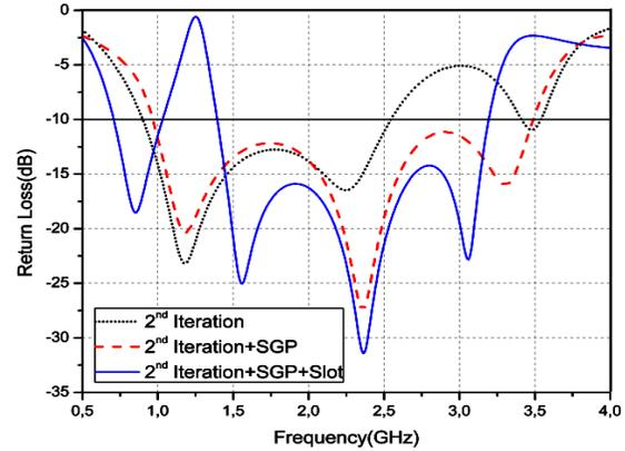
Fig. 5  $S_{11}$  curves for different configurations of the antenna.
