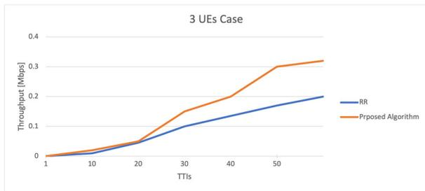
Fig. 4 Overall Cell Throughput in 3 UEs Scenario.
