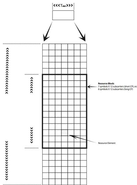
Fig. 2 The Radio Resource Block [10].
