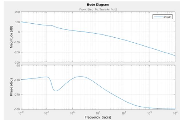
Fig.7 Bode diagram after the process of optimizing the controller settings
