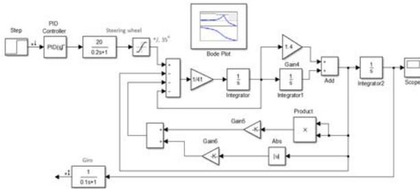
Fig.5 Schematic of the open loop stabilization system (for the synthesis of the PID controller)
