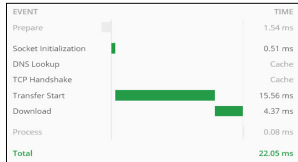
Figure 10: The execution time of an authorized Get request using the mechanism.
