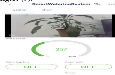
Figure 9: Blynk interface when soil moisture in wet case
