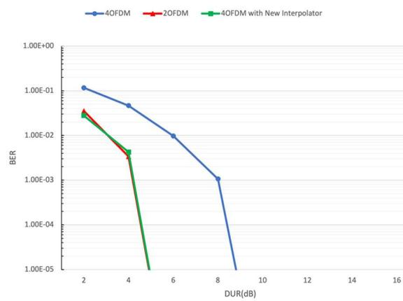
Fig. 12 : BER vs DUR (dB), QPSK
