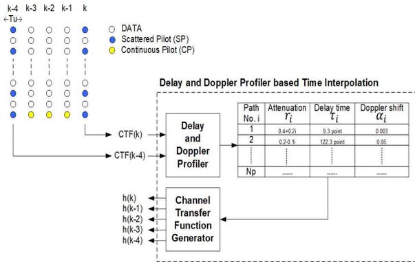
Fig. 8: Detail of Delay and Doppler interpolator
