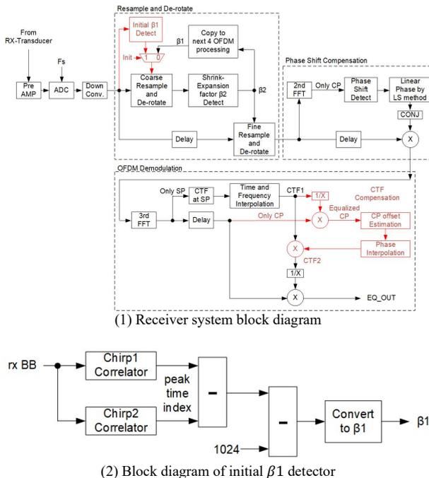
Fig. 3: Proposed receiver system block diagram with (1) receiver system and (2) block diagram of initial  $\beta_1$  detector
