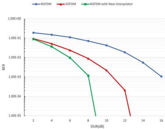
Fig. 13 : BER vs DUR (dB), 16QAM
