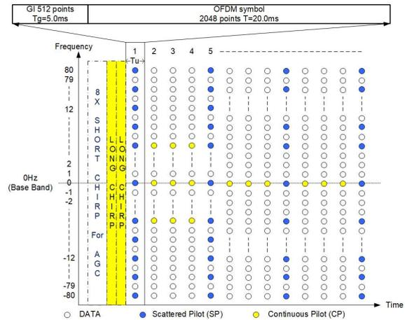
Fig. 4: Time-Frequency structure of OFDM that is inserted SP
