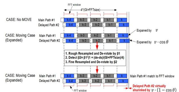
**Fig. 7:** Delayed Path with Doppler Shift
