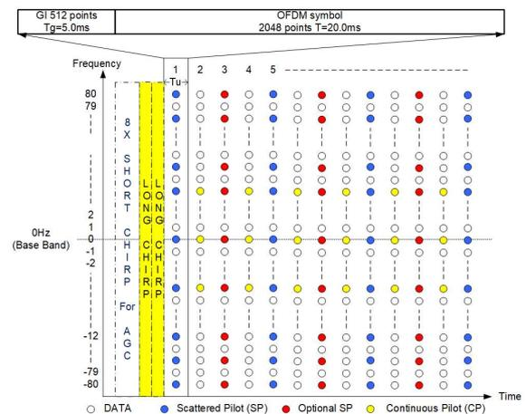
Fig. 5: Time-Frequency structure of OFDM that is inserted SP
