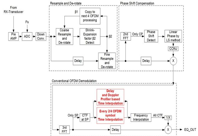
**Fig. 6:** Detail of receiver block diagram
