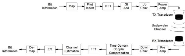
Fig. 2: OFDM block diagram
