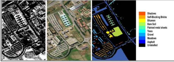
Figure 4: Original image and Ground Truth of Pavia University dataset
