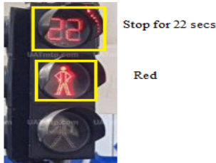
Figure 8: Detected traffic signal and timer
