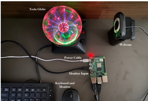
Figure 8. General view of the webcam sensor system.
