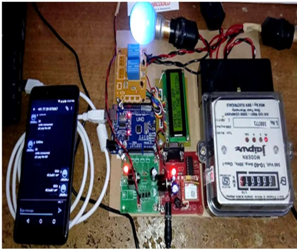
Fig.5. Hardware implementation of Android Mobile App based energy monitoring system
