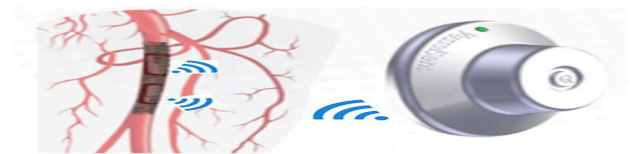
Figure 1. An example of a self-monitoring vascular stent developed by Vesselsens, capable of two-way communication to enable predictive medical interventions for restenosis.
