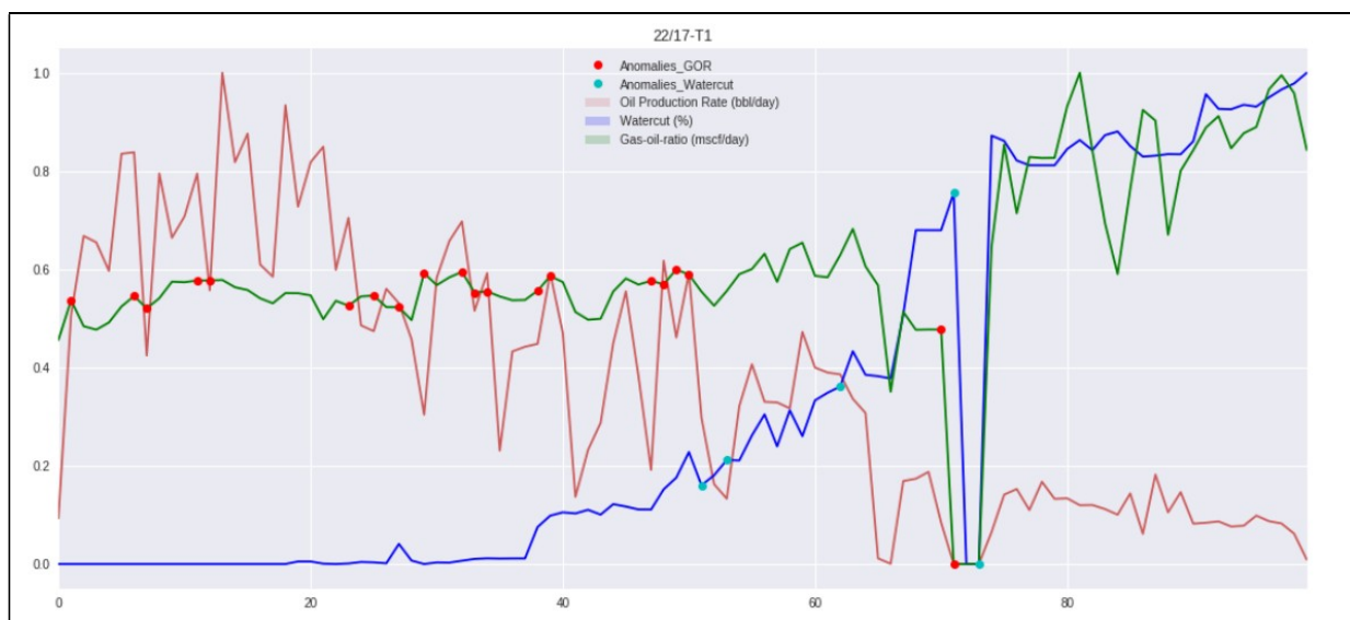
Fig. 6 Anomaly detection (statistical based) on well 22/17-T1 (Arbroath section)
