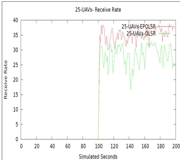
Figure. 6. 25-UAVs- Receive Rate (kbps) Using EP OLSR vs. OLSR
