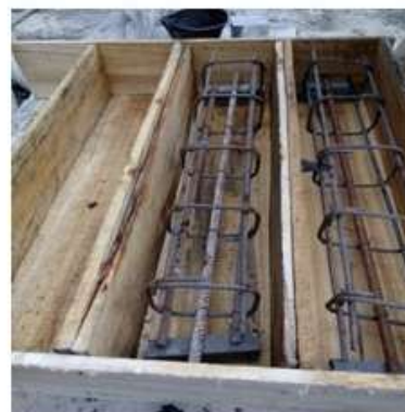
Figure 2: How to formatting and reinforcement the sample Figure 3: Cross-axis rebar (s) placement inside the cores with 10cm of diameter
