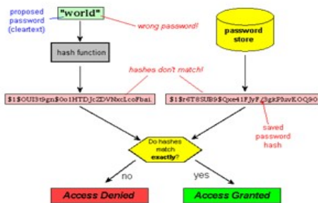
Figure2: User authentication using the hash function
