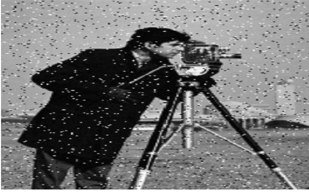
Figure 8 Image corrupted with salt and pepper (Impulsive) noise.
