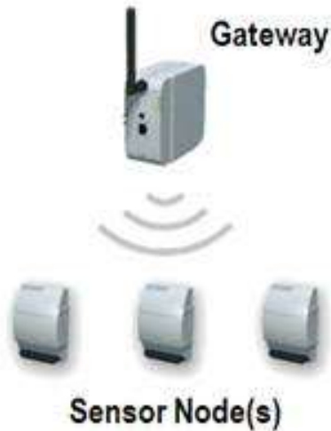
Figure.2 WSN Components, Gateway, and Distributed Nodes
